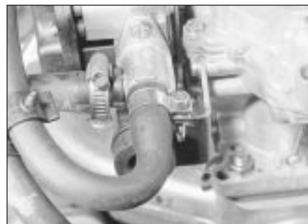
12.6a Automatic choke coolant pipe connection . . .
