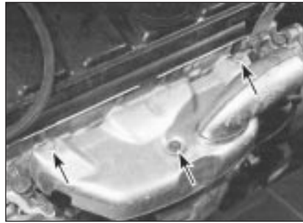
15.2 . . . then undo the three retaining screws (arrowed) and remove the exhaust manifold shroud (TU engine)
