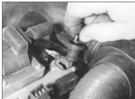
2.4 Undo the intake duct front bolt then release the rear fastener, and remove the duct and hose assembly (TU engine)
