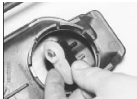
3.14c . . . then withdraw the vacuum switch from inside the duct
