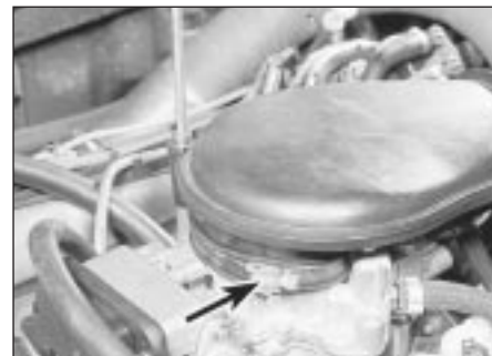
2.5 On the XU engine unscrew the bolt securing the air inlet duct, then loosen the clip
