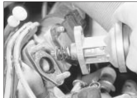
4.5 Removing the fuel pump (XU engine)
