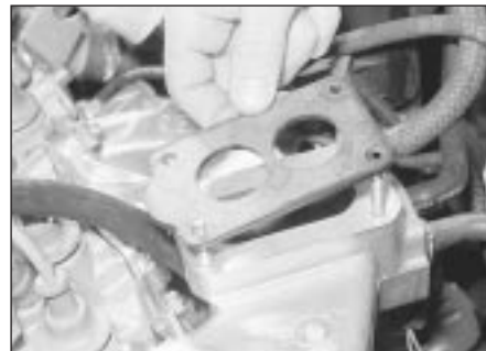
12.11 Removing the insulating spacer
