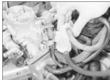
12.9 Lifting off the fuel reservoir
