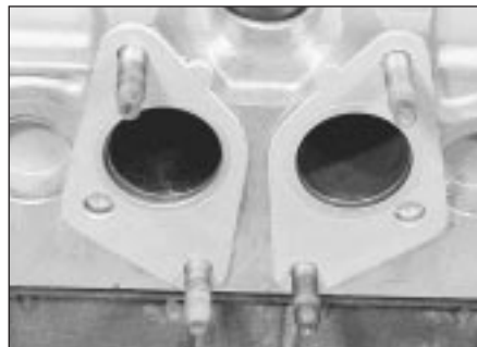
15.7 New gaskets fitted to the exhaust ports on the cylinder head (XU engine)
