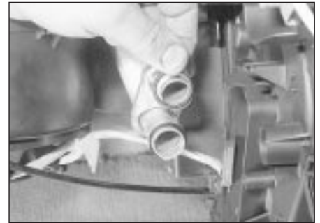
9.36c . . . and recover the O-rings from the pipe connections
