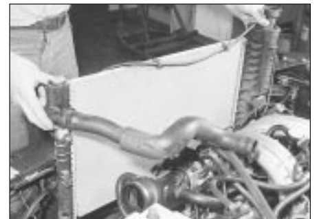
3.11 Lifting out the radiator
