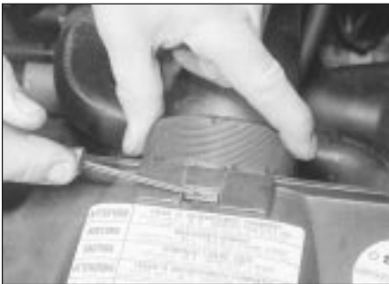
3.5a Depress the securing clip . . .
