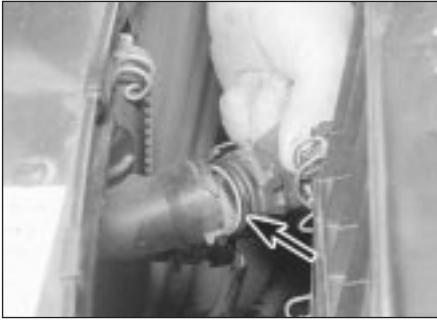
2.12b Recover the O-ring (arrowed) from the end of the hose connector
