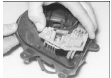
9.68b . . . and withdraw the control module
