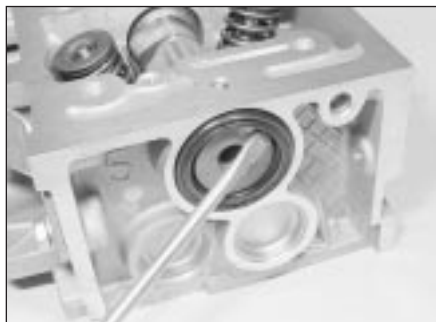
10.9a . . . prise out the oil seal . . .
