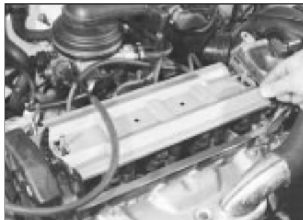
4.6b . . . and remove the oil baffle plate
