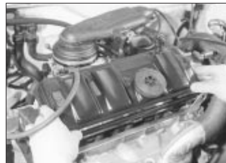
4.5 . . . and lift off the cylinder head cover
