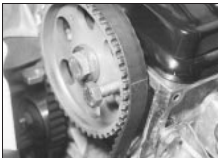
3.5 . . . then insert a 10 mm bolt through the cam sprocket timing hole, and locate it in the cylinder head
