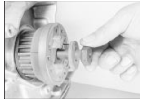
7.11a Remove the crankshaft sprocket retaining bolt . . .
