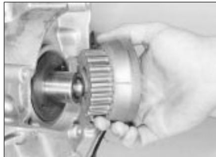
7.11b . . . then slide off the sprocket
