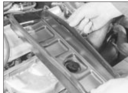
4.8 On refitting, ensure the rubber seal is located on the cylinder head cover
