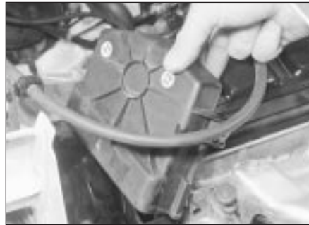
5.1b . . . and remove the upper timing belt cover
