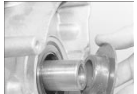
7.12 Remove the flanged spacer if necessary
