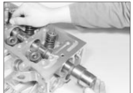
10.9b . . . and slide out the camshaft
